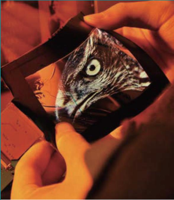
FlexUPD's flexibility allows for two-sided surface visibility for display or non-display products.
