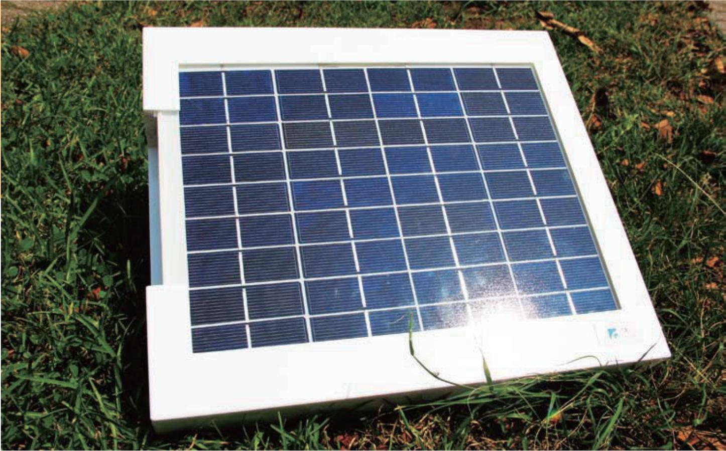
ITRI's green energy antenna technology has successfully integrated antenna transmission and solar panel power storage technology.
